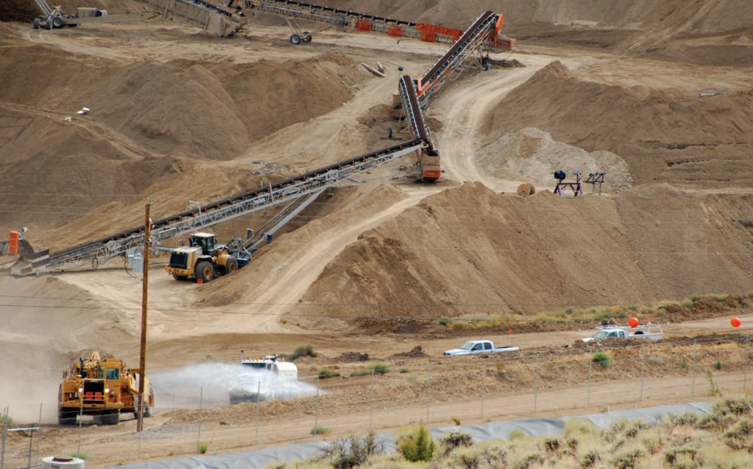
A series of conveyor belts carries mineral-rich ore to the top of Comstock Mining's heap leach pad. The leach pad currently processes 1 million tons of mineral-rich ore per annum (year).
