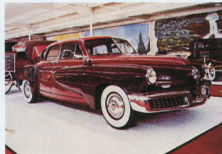
The center headlight on this rare 1947 Tucker turns left and right with the steering wheel. It was an idea that didn't catch on.
